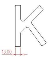
Dimensions are used to restrict geometry.
